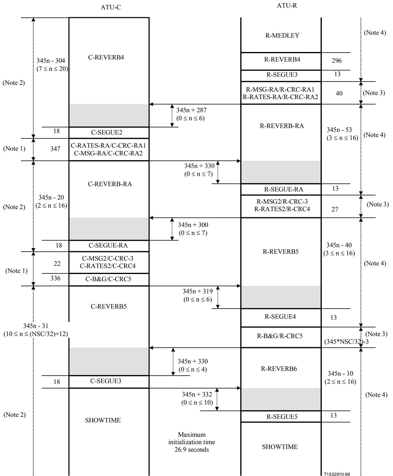
NOTE 1 – The ATU-C shall transmit the FEXTR symbols, and shall not transmit as NEXTR symbols except the pilot tone.
