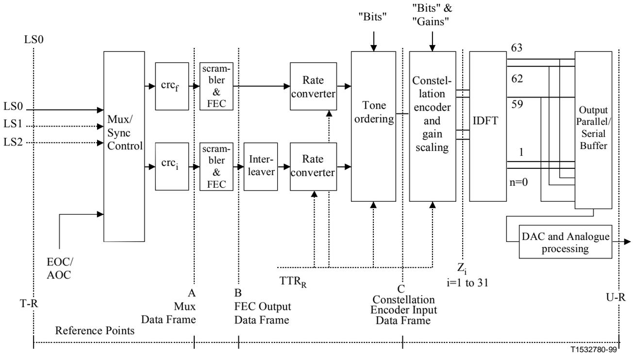
NOTE – The TTR<sub>R</sub> shall be generated in ATU-R from the received TTR<sub>C</sub> signal, and it is locked to 690 periods of upstream sampling clock (276 kHz).
