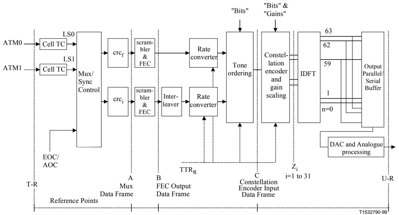
NOTE – The  $TTR_R$  shall be generated in ATU-R from the received  $TTR_C$  signal, and it is locked to 690 periods of upstream sampling clock (276 kHz).
