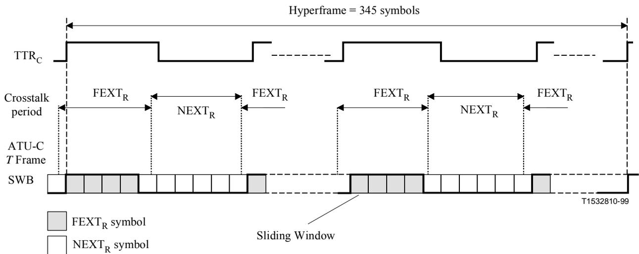
Figure Q.6/G.992.1 – Sliding window for downstream symbols
